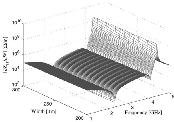
Fig. 3. Magnitude of  $\partial Z_{11}/\partial W$  for  $h = 450 \mu\text{m}$ .
