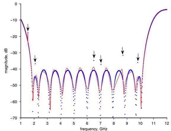
Fig. 2 Magnitude of  $S_{11}$ : model  $L_2$  (solid curve) and data (dots)
