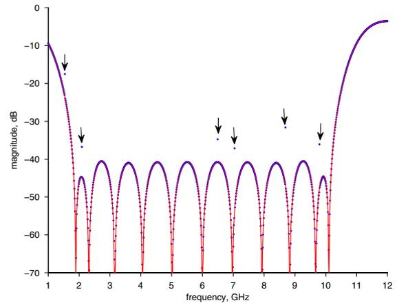
Fig. 1 Magnitude of  $S_{11}$ : model  $L_1$  (solid curve) and data (dots)
