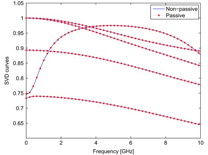
Fig. 4. Balun: singular value curves of passive and nonpassive model.
