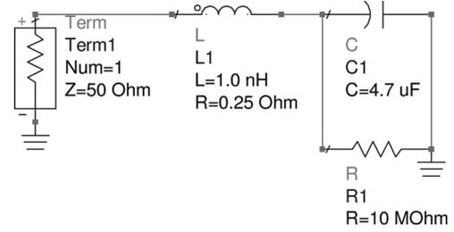
Fig. 1. Shunt capacitor: schematic.
