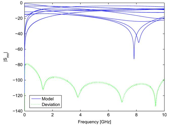
Fig. 8. Balun: singular values passive dc-compliant macromodel and deviation.
