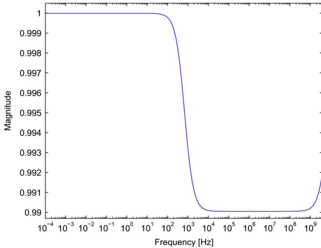
Fig. 2. Shunt capacitor: magnitude of  $S$ -parameters.
