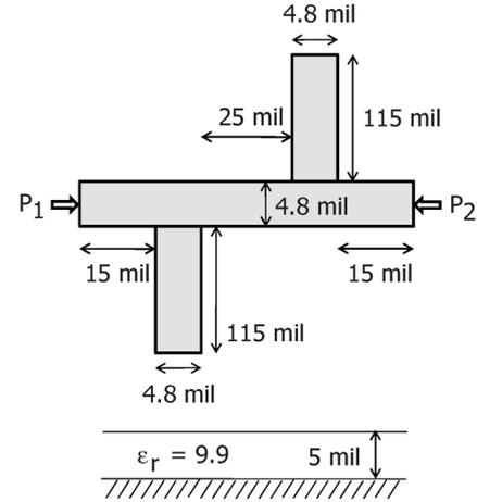
Fig. 2. Structure of the microwave filter.
