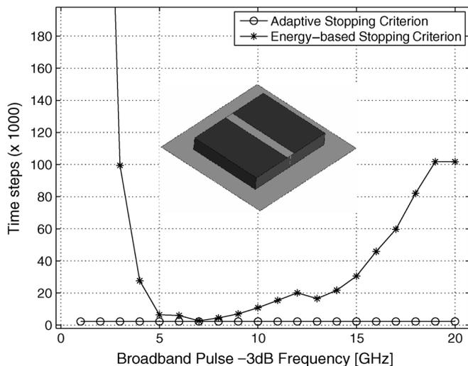
Fig. 5. Number of time steps needed vs. frequency content of input pulse.
