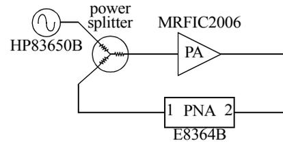
Fig. 1. Scheme of the measurement setup
