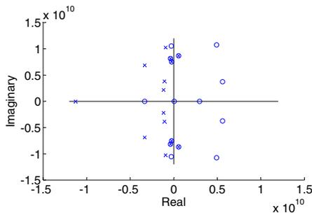
Fig. 6. The parametric model  $\hat{G}$  ( $M_b = M_a = 15$  and  $N_b = N_a = 8$ ), evaluated for an input power of 3.4dBm, has been parametrized in pole (represented by a cross) and zero (represent by a circle) locations. It is clear that this model is not stable for this power slice. Furthermore one can notice that the unstable pole can be cancelled by a zero, indicating the model order can be lowered.
