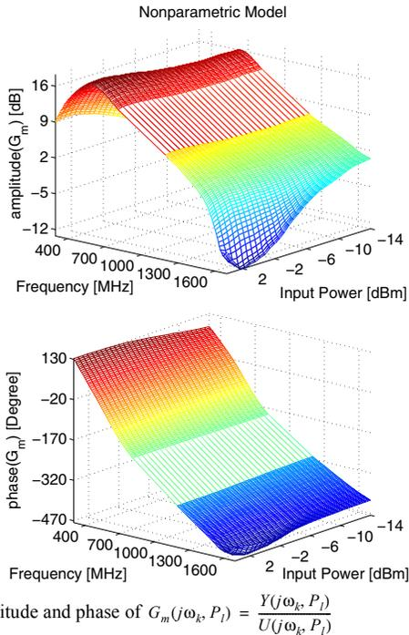
Fig. 3. Amplitude and phase of  $G_m(j\omega_k, P_l) = \frac{Y(j\omega_k, P_l)}{U(j\omega_k, P_l)}$
