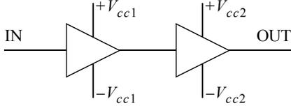
Fig. 2. Supply voltages of the Motorola MRFIC2006
