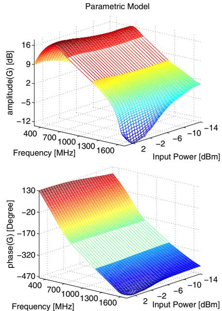
Fig. 4. Amplitude and phase of the estimated 2D rational (parametric) model  $G(j\omega, P, \hat{\theta})$
