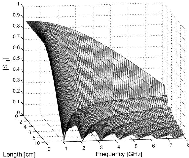
Fig. 2. Reflection coefficient  $S_{11}$  of macromodel using first order derivatives.
