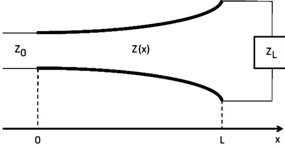
Fig. 1. Exponential tapered transmission line [16].
