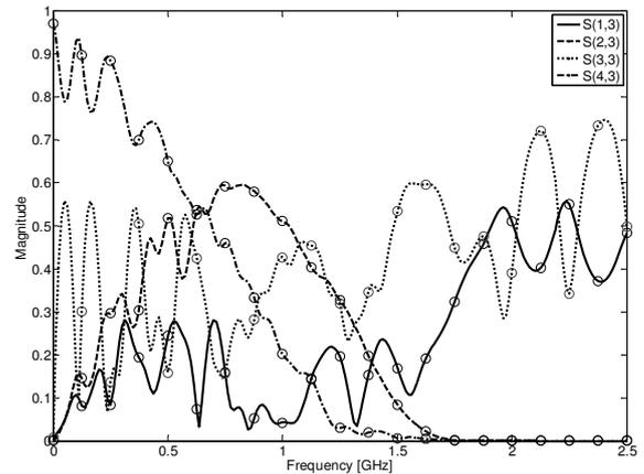
Figure 7: RDRAM channel: magnitude of the measured data (drawn as lines) and macromodel (indicated with markers).
