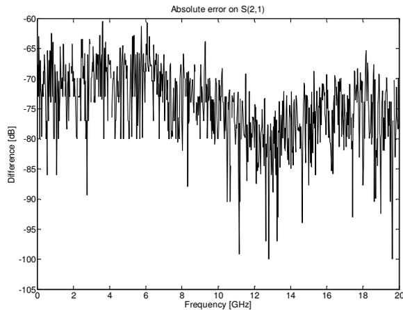
Figure 5: Coupled microstrips: difference between macromodel and measured data of the transmission parameter  $S(2,1)$ .
