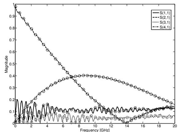
Figure 4: Coupled microstrips: magnitude of the measured data (drawn as lines) and macromodel (indicated with markers).
