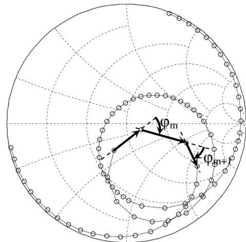
Figure 1: Calculating the cumulative phase variation along the data path, with increasing frequencies.
