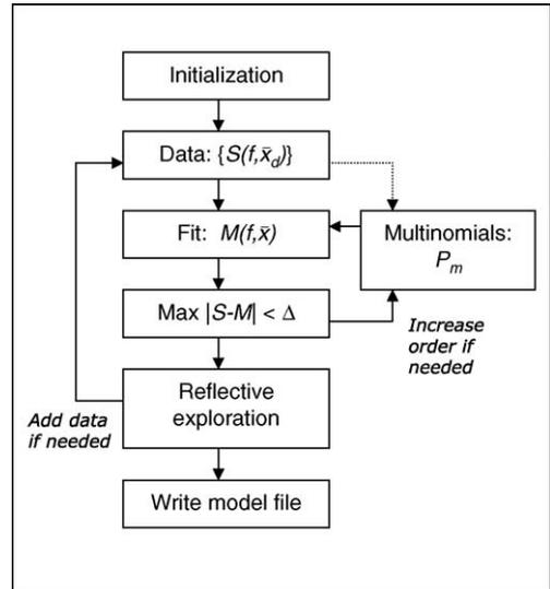
Fig. 1. Adaptive modeling and sampling flowchart.
