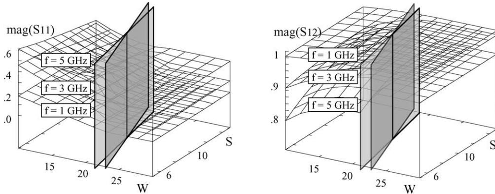
Fig. 8.  $S$ -data of spiral as a function of  $f$ ,  $W$  and  $S$ .
