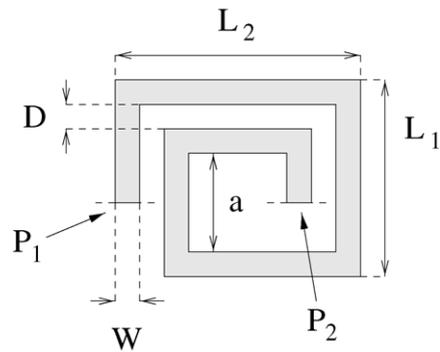
Fig. 3. Layout of spiral inductor.
