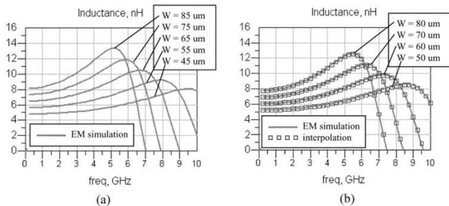
Fig. 9. (a) Simulated inductance for different values of the layout parameter. (b) Interpolated inductance for intermediate values of the layout parameter.
