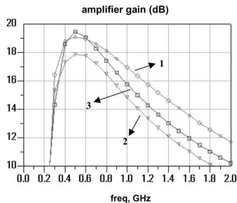
Fig. 10. Amplifier gain as a function of frequency for the amplifier of Fig. 3 (1: original schematic ( $\circ$ ), 2: result including board parasitics ( $\nabla$ ), 3: result after optimization ( $\square$ )).
