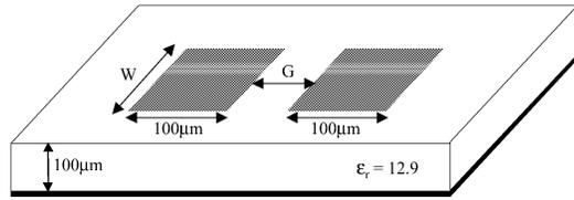
Fig. 12. Microstrip gap on a GaAs substrate.
