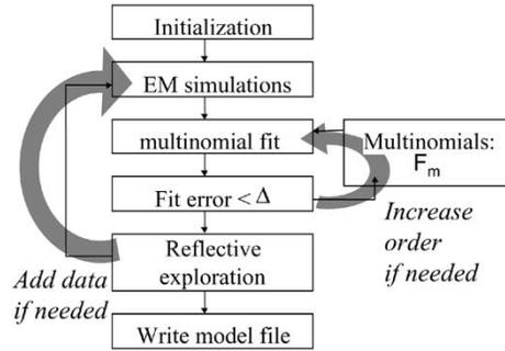
Fig. 11. Flowchart of the up-front generation of a MAPS-EMDB model of a generalized layout component.
