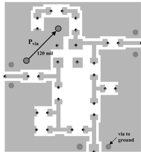
Fig. 4. Footprint of the RF board layout for the LNA of Fig. 3.
