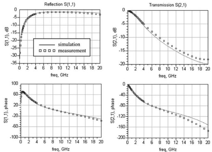
Fig. 7. Simulated and measured two-port  $S$ -parameter data for the spiral inductor with  $W = 65 \mu\text{m}$ .
