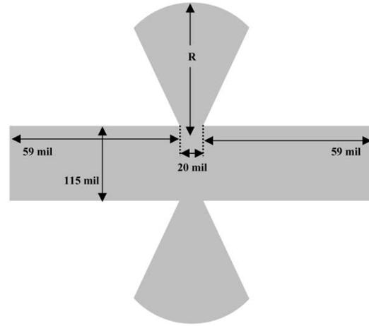
Fig. 14. Top view of the layout of a butterfly capacitor.
