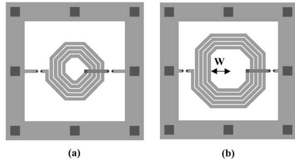
Fig. 6. Layout of a four-turn octagonal silicon spiral inductor. (a)  $W = 45 \mu\text{m}$ . (b)  $W = 85 \mu\text{m}$ .
