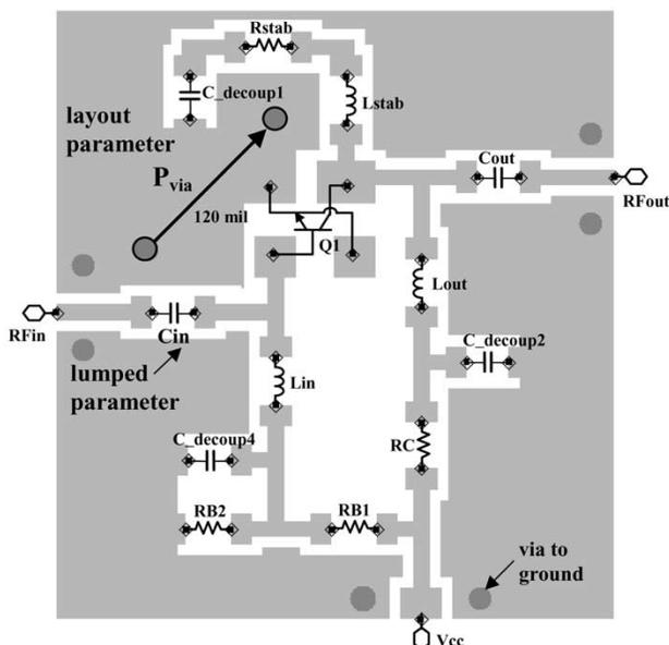
Fig. 5. Schematic of the LNA including the GLC for the RF board footprint, as depicted in Fig. 4.
