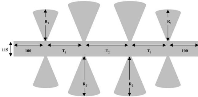
Fig. 17. Total filter layout corresponding to the circuit equivalent of Fig. 16 (all dimensions are in mils; microstrip substrate with thickness 59 mil and  $\epsilon_r = 4.3$ ).
