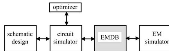
Fig. 2. Block diagram of the EM-circuit co-optimization environment showing the EMDB.
