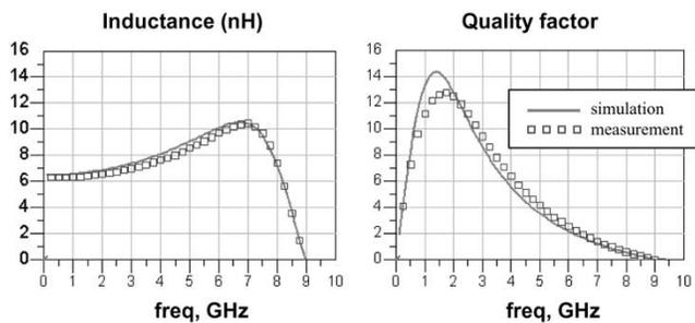
Fig. 8. Simulated and measured inductance value and quality factor for the spiral inductor with  $W = 65 \mu\text{m}$ .
