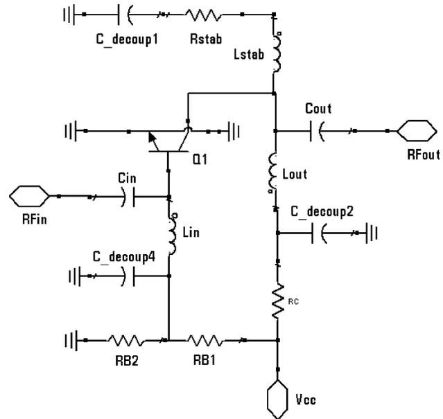
Fig. 3. Schematics of an LNA.
