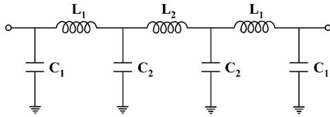
Fig. 16. Circuit equivalent of the seventh-order Chebyshev filter.
