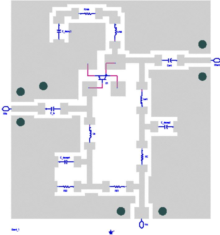
Schematic of the low noise amplifier including the GLC for the RF board footprint
