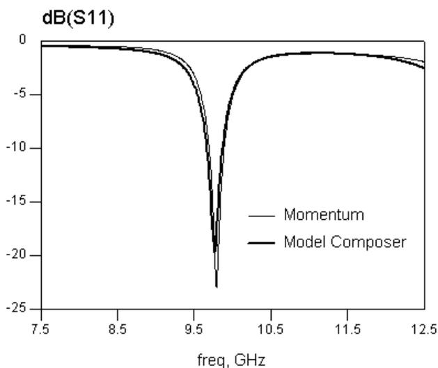
Figure 5:  $S_{11}$  of Slot-coupled microstrip-fed patch antenna
