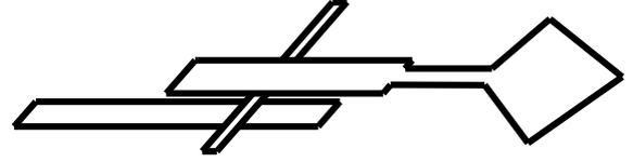
Figure 2: Slot-coupled microstrip-fed patch antenna structure
