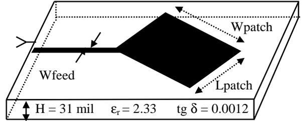
Figure 3: Layout of corner-fed patch
