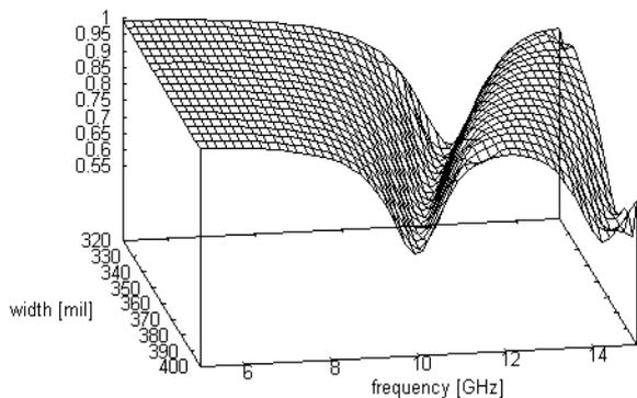
Figure 4:  $S_{11}$  of corner-fed patch ( $W_{feed} = 8$  mil)
