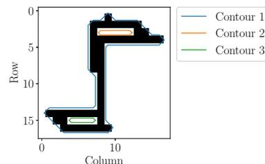
Fig. 3: The identification of the VI trajectory contours of a CFL. Only the outer contour is used for object classification.
