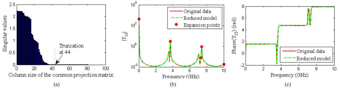
Fig. 3. (a) Singular values of the common projection matrix, (b) magnitude of  $Y_{13}$  with the expansion points and (c) phase plot of  $Y_{13}$ .
