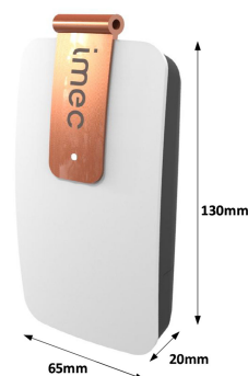
Fig. 2. ROBIN device used in this study. It is a compact wearable with minimal discomfort for the patient. The device is worn around the neck and is attached to the chest via adhesive stickers.
