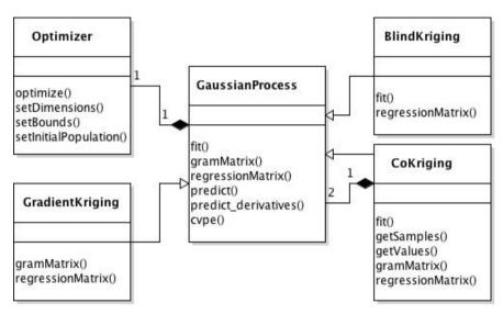
Figure 1: The UML class diagram of the ooDACE toolbox.
