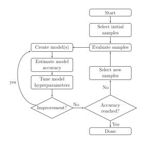
FIG. 4. Flowchart of the SUMO toolbox workflow.
