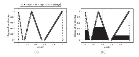
FIG. 1. Figure (a) shows the output membership functions low, average, and high for S. In (b), the clipped functions for the example with input membership degrees of 0.5 in  $C_{high}$ , 0.15 in  $A_{low}$ , and 0.45 in  $A_{high}$  are shown. The vertical line indicates the weight obtained by defuzzification of the resulting output membership distribution by the centroid method.
