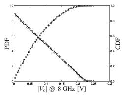
Fig. 8: PDF and CDF of the magnitude of the common-mode voltage  $V_c$  at 8 GHz for the unbalanced differential IEM lines. Full black line: PDF computed using the novel technique; Dashed black line: CDF computed using the novel technique; Circles ( $\circ$ ): PDF computed using MC technique; Squares ( $\Box$ ): CDF computed using MC technique.
