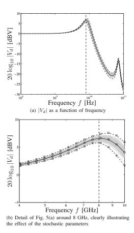
Fig. 5: Bode plot of the magnitude of the differential voltage  $V_d$  for the unbalanced differential IEM lines. Full black line: mean  $\mu_{|V_d|}$  computed using the novel technique; Dashed black line:  $\pm 3\sigma_{|V_d|}$ -variations computed using the novel technique; Gray lines: 100 samples from the MC run; Circles ( $\circ$ ): mean  $\mu_{|V_d|}$  computed using MC technique; Squares ( $\Box$ ):  $\pm 3\sigma_{|V_d|}$ -variations computed using MC technique.
