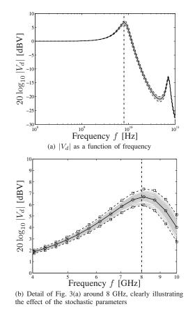
Fig. 3: Bode plot of the magnitude of the differential voltage  $V_d$  for the balanced differential IEM lines. Full black line: mean  $\mu_{|V_d|}$  computed using the novel technique; Dashed black line:  $\pm 3\sigma_{|V_d|}$ -variations computed using the novel technique; Gray lines: 100 samples from the MC run; Circles ( $\circ$ ): mean  $\mu_{|V_d|}$  computed using MC technique; Squares ( $\Box$ ):
