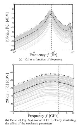
Fig. 6: Bode plot of the magnitude of the common-mode voltage  $V_c$  for the unbalanced differential IEM lines. Full black line: mean  $\mu_{|V_c|}$  computed using the novel technique; Dashed black line:  $+3\sigma_{|V_c|}$ -variation computed using the novel tech-
