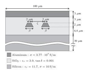
Fig. 1: Cross-section AA' (see Fig. 2) of the differential IEM lines (not on scale).
