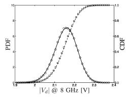
Fig. 4: PDF and CDF of the magnitude of the differential voltage  $V_d$  at 8 GHz for the balanced differential IEM lines. Full black line: PDF computed using the novel technique; Dashed black line: CDF computed using the novel technique; Circles ( $\circ$ ): PDF computed using MC technique; Squares ( $\Box$ ): CDF computed using MC technique.
