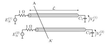
Fig. 2: Source-line-load configuration. The cross-section AA' is depicted in Fig. 1.
