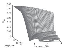
**Fig. 2** *Reflection coefficient*  $S_{11}$  *for*  $\varepsilon_r = 4$
