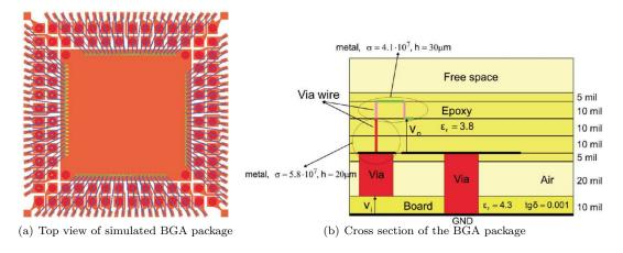
Figure 1: Simulated BGA Package
