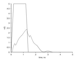
Fig. 1 Transient results (black line = 'measured' output) (dashed line = output from reduced model)
