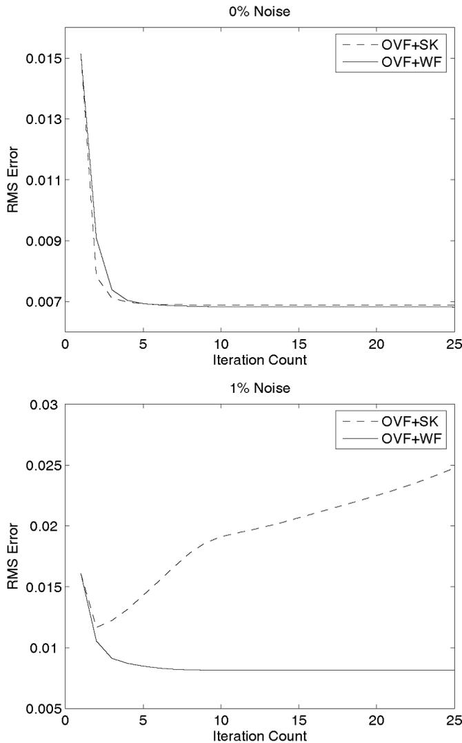
Figure 1: RMS Error as function of Iteration Count - 0% Noise (upper) 1% Noise (lower)
