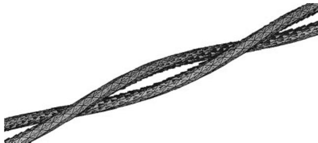
Figure 1. Schematics of a two-conductors unshielded twisted cable with a typical mesh for SURFCODE simulation.
