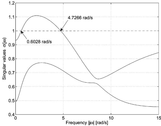
Fig. 2. Singular values of  $S(j\omega)$  and crossover frequencies using  $\bar{M}_P$ .
