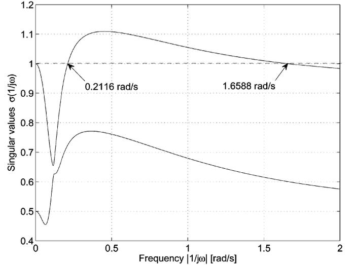
Fig. 1. Singular values of  $S(1/j\omega)$  and crossover frequencies using  $\bar{M}_P$ .
