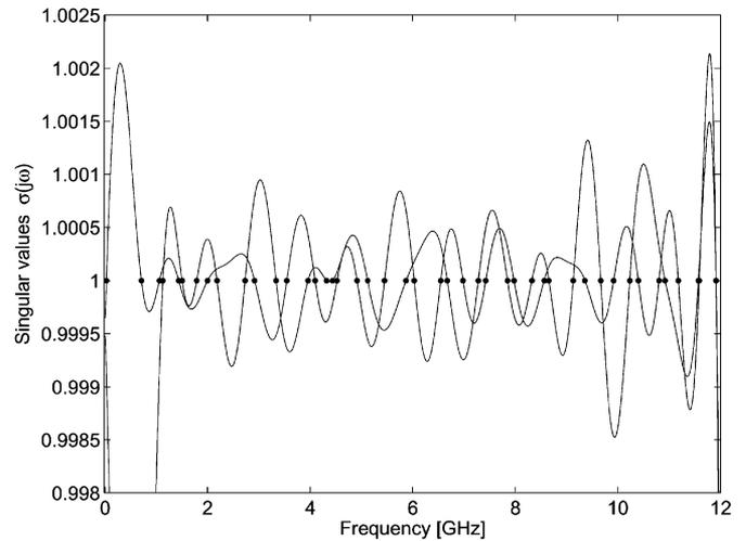
Fig. 4. Singular values of  $S(j\omega)$  and crossover frequencies using  $\bar{M}_P$ .
