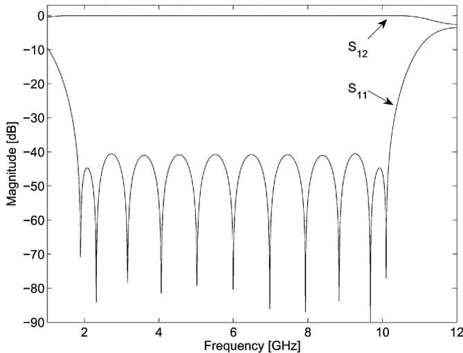
Fig. 3. Magnitude of scattering matrix elements  $S_{11}$  and  $S_{12}$ .
