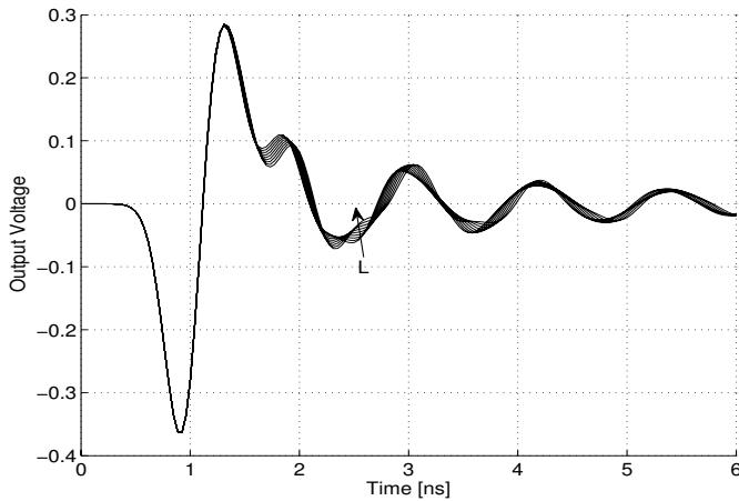
Figure 2: Output voltages for various values of length L
