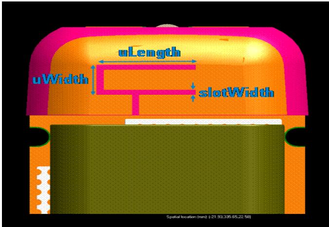
Figure 1: Non-Planar Inverted-F Antenna
